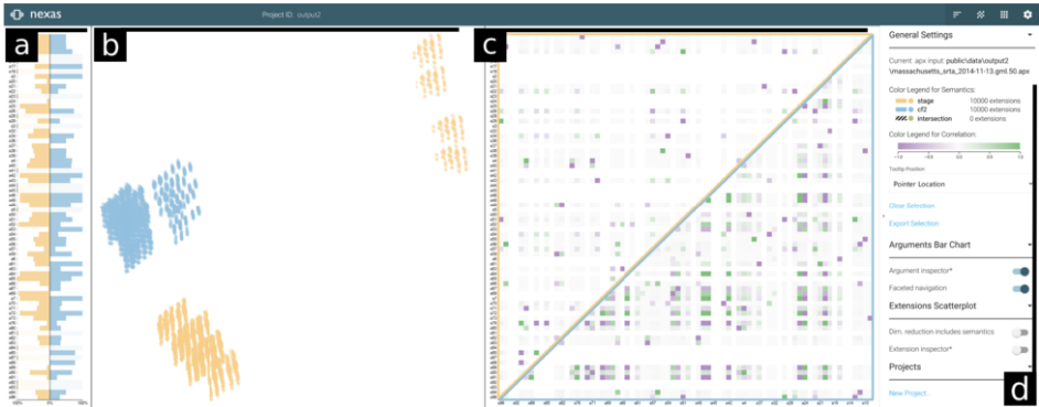
Figure 1. NEXAS interface showing a) the Argument View : bar chart with the relative frequencies of the arguments by semantics, b) the Extension View : scatterplot with the dimensionality reduced solution space, c) the Correlation View : correlation matrix of accepted arguments wrt. two semantics separated by the diagonal, and d) a sidebar with the color legend, settings and inspection options.
